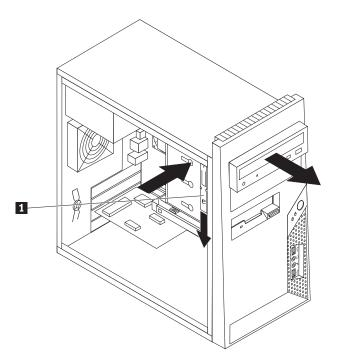
Figure 27. Removing the optical drive
